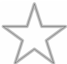
The drawing represents the actual path taken by the centreline of the tool, and the tool does not have an infinitely small diameter, so the finished result will be a bit smaller than it was actually drawn. The difference is half the diameter of the cutter used and as we wanted the star to have precise dimensions the result can be scrapped.
